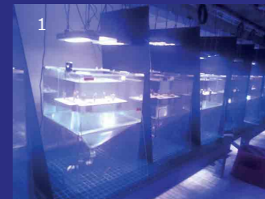
Figure 1: Experimental set up – 16 tanks, 4 light treatments, black dividers to reduce light spillover.
